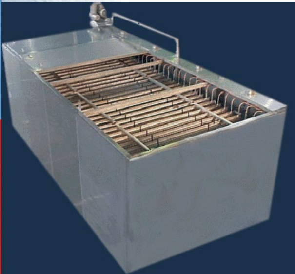
PIC (LEFT TO RIGHT): Panelsystems in a tank, with air agitation to increase heat transfer and reduce fouling effects; Ready to plug cooling system with refrigeration units: (up to 20 kW)
