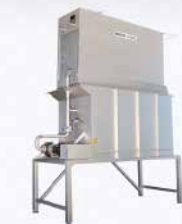
Melting through for wax, with round corners at edges and collars
